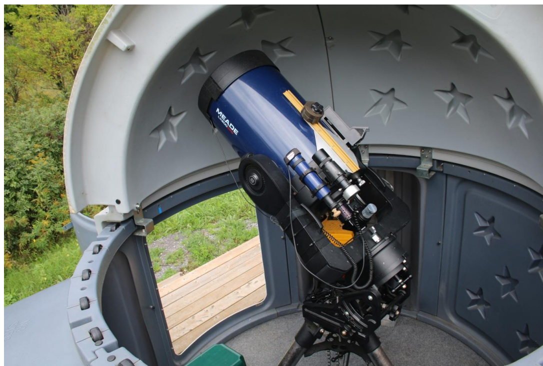
The Meade 14" SCT with autoguider and Telrad installed (photo by Paul Klauninger)
